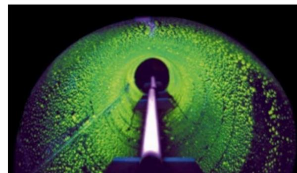
Ducting sprayed with riboflavin and lighted with UV light
